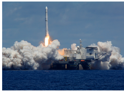
Images: Sea Launch. Platform is converted oil rig.
